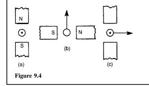
The direction of the e.m.f., and thus the current due to the e.m.f. may be obtained by either Lenz's law or Fleming's Right-hand rule (i.e. GeneRator rule).
